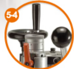
5-4 主軸微調距離 Precise fine tuning and securing arrangement
